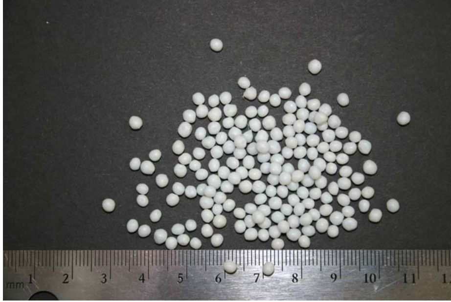
Figure 3.17. The polyester scalene ellipsoids as used in the rheological experiments. The ellipsoids have a specific gravity of 1.40 and have an equivalent spherical particle diameter of 2.93 \pm .02 mm. The ruler shown for reference measures in centimeters.
