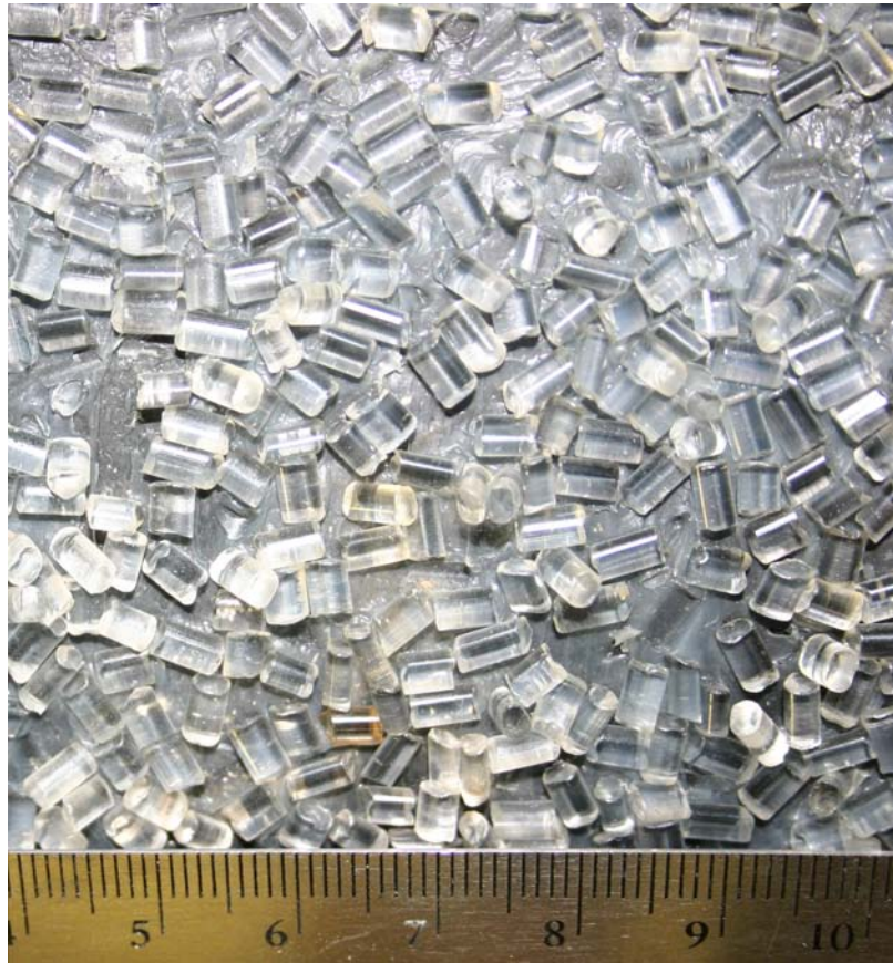
Figure 6.4. Photograph of the surface roughness added to inner and outer cylinders. The surface volume fraction is 0.70. Markings on the ruler are in centimeters.
