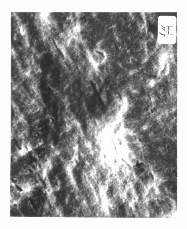
SEM at 8400% of uranium target which has been sputtered by 3 x  $10^{17}$  80 kev Ar<sup>+</sup> ions per cm<sup>2</sup>. (see p.28)
