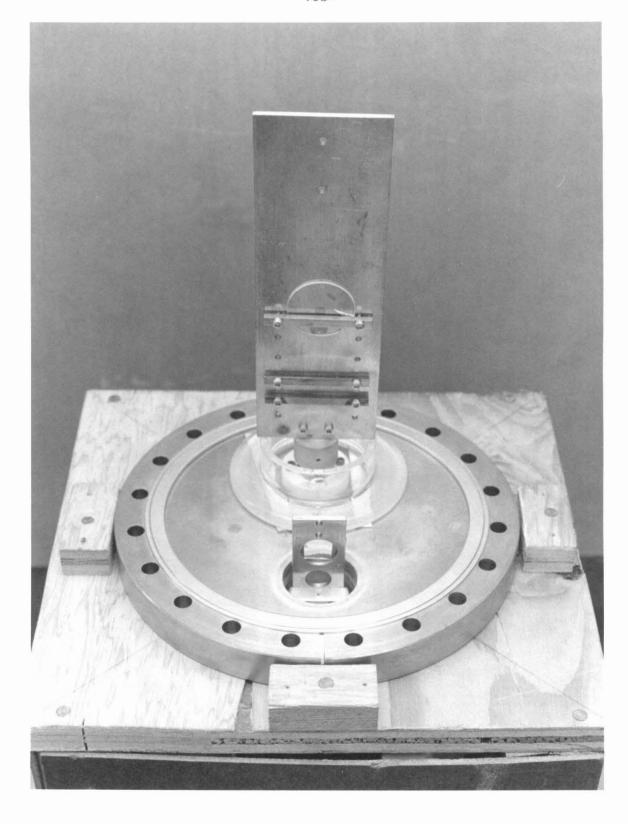
Collimation cylinder added to assembly. (see p.12)
