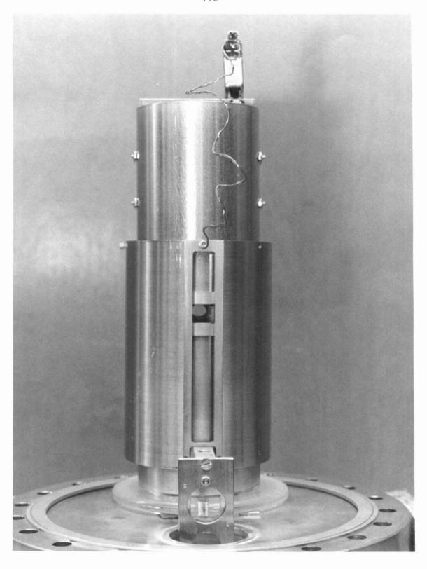
The ultra-high vacuum system. (see p.12) Essential components are sketched in Fig. 10. The entire assembly may be adjusted vertically and horizontally for purposes of alignment to ion beam.
