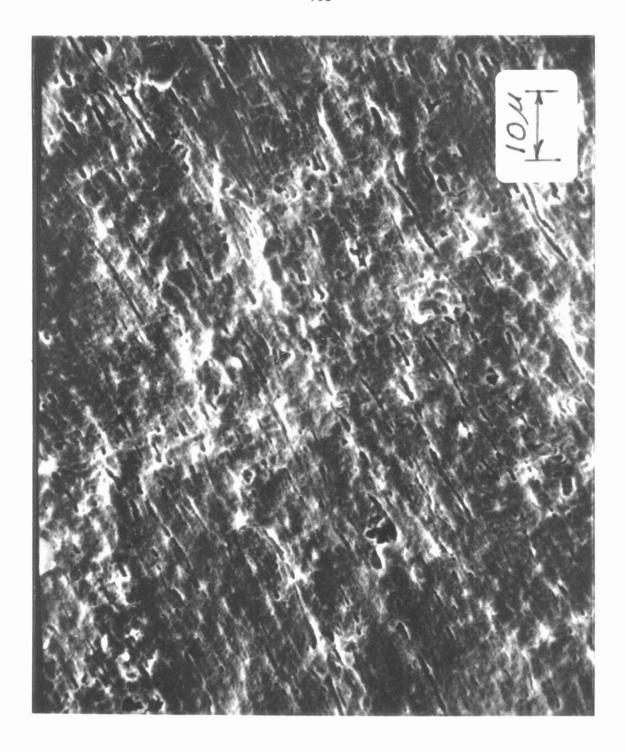
Scanning electron micrograph at 800% of uncleaned uranium target. (see p. 29)
