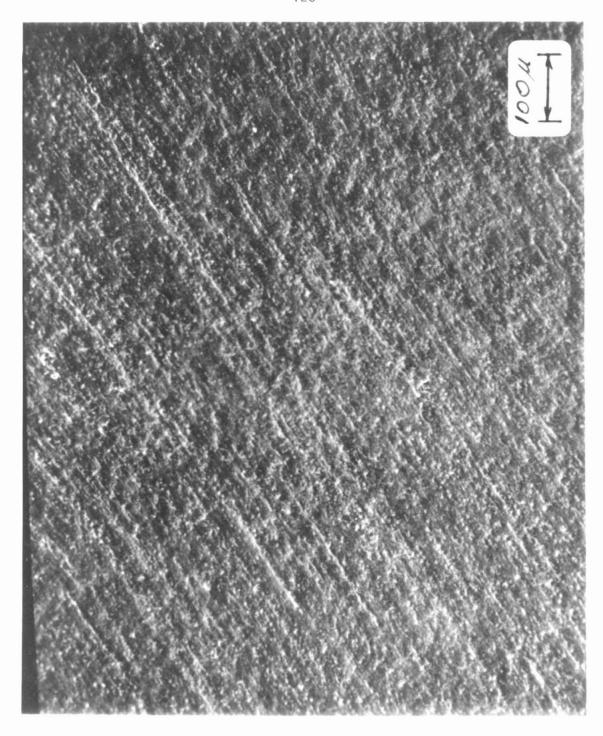
SEM of uranium target at 2400X. (see p.28) This area of target has not been sputtered, but was cleaned in  ${\rm HNO_3}$ .
