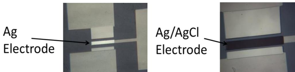
Figure 25 : Silver based integrated Reference Electrodes
