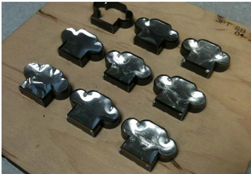
*Figure 5.1 Dies for Metal Cutting*
