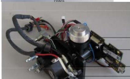
Combined temperature control and real time fluorescence imaging module used in the qNAT instrument
