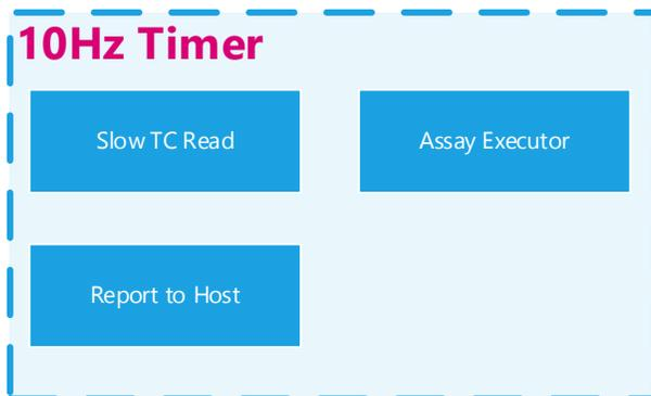
A 10Hz timer with pre-emptive execution is used for assay execution to count the step times, sampling temperature from Thermocouples and for reporting to host.
