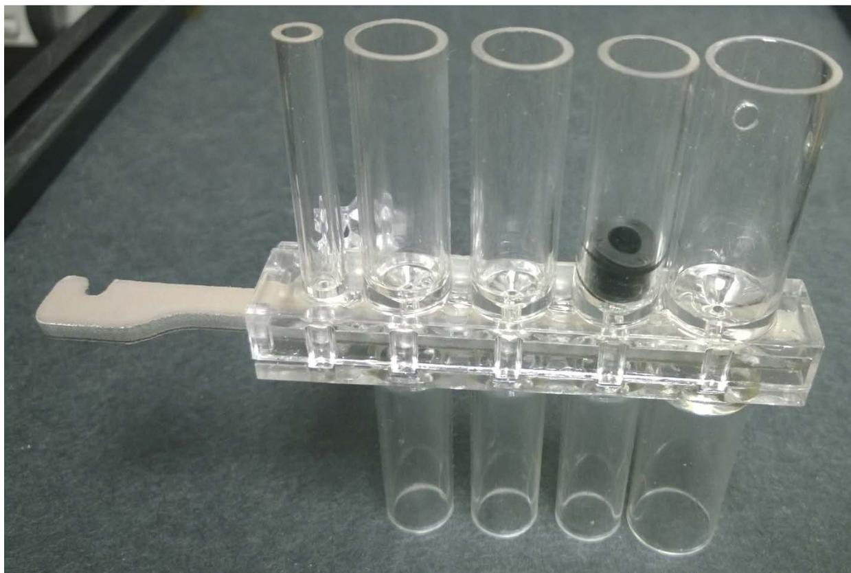
*Figure 9.7 Injection Molded Cartridge*
