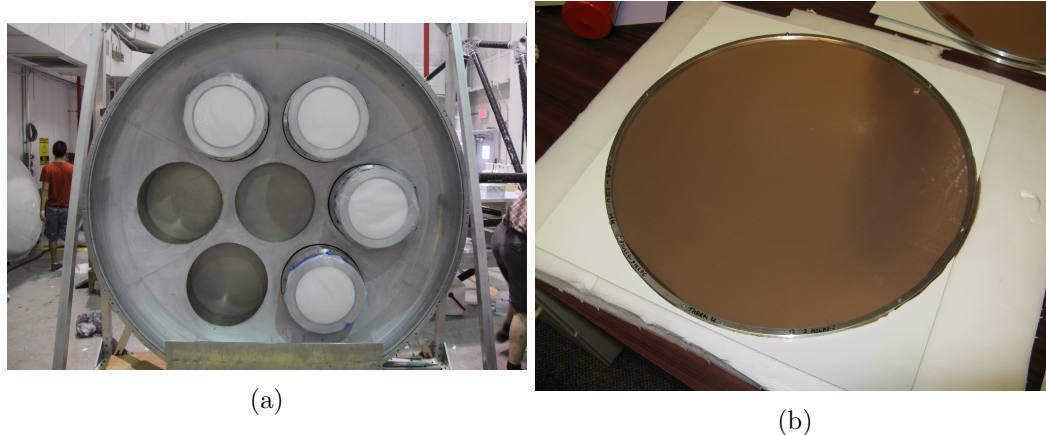
Figure 2.9: Left : Flight windows installed in the top dome of the flight cryostat. Photo courtesy of Steve Benton. Right : A close-up of one of the IR shaders.
