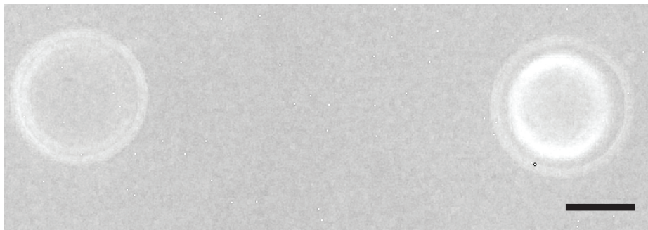
Figure 5.2: Demonstration that proteins are successfully bound to the surface of the microtoroid. These fluorescent microscope images show FITC-Fc bound to a linker bound to the surface of the microtoroid (top view). The images are of the same sample, just taken at different magnifications. The white glow is from the FITC and indicates that the protein is present on the toroid's surface. Scale bars are 45\ \mu\text{m} .
