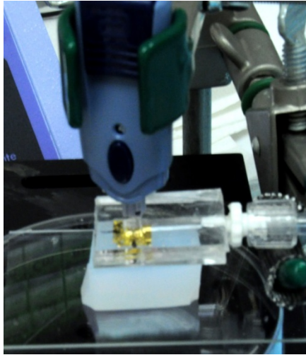
Figure 5.5- Impact Penetration Setup. Lancing device sits above the Syringe Pump Skin Patch. Upon actuation, microneedles are driven into hydrogel (4% agarose) as a laboratory model for skin.
