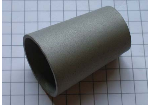
Figure 7.2: Photograph of the 10 \mu\text{m} media grade porous injector section against a 6.35 mm grid. See also Figure 7.1.
