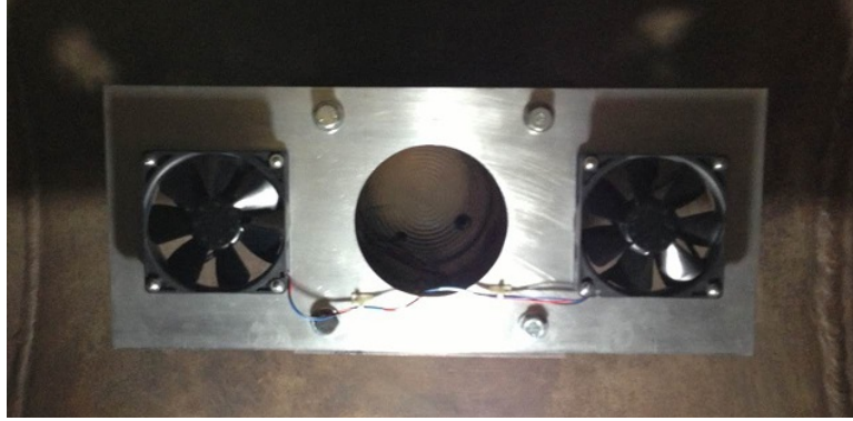
Figure 2.4: Gas premixing tank internal fans.
