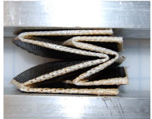
Figure 7.18: Tapered Miura-ori conical shell manufactured in the laboratory, in different stages of deployment.
