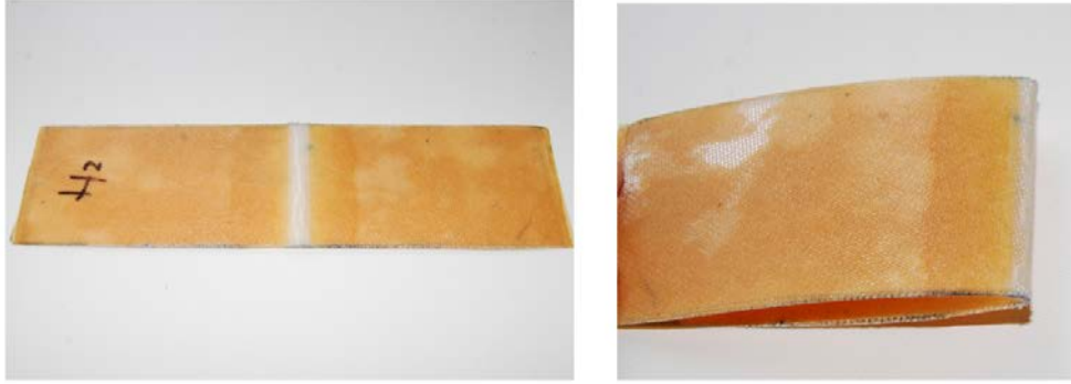
Figure 6.12: Astroquartz dual-matrix laminate with silicone hinge, unfolded and folded.
