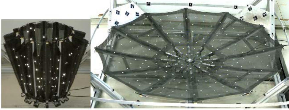
Figure 1.4: SMART (Shield-membrane antenna reflector technology) demonstrator, taken from [14]. The reflector is made of triaxial weave carbon fiber-reinforced silicone.
