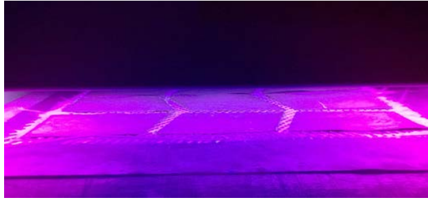
Figure 6.7: UV curing of the silicone. The epoxy film paper acts as a mask so that the silicone only cures in the exposed area. The curing time is less than one minute.
