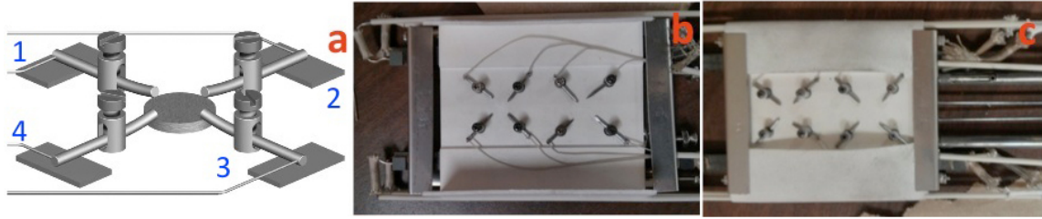
Figure 2.2. Sample holder of the Hall effect and resistivity measurement setup, a) schematic of sample and measurement geometry, b) c) picture of sample holder without and with insulation.
