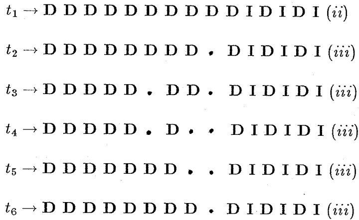
Fig. 4.4 State of repeaters in blocking condition (iii)
