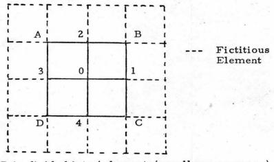
The plate ABCD is divided into 4 elements (usually many more). Fictitious elements are introduced to apply the boundary conditions. Fig. 9.1
