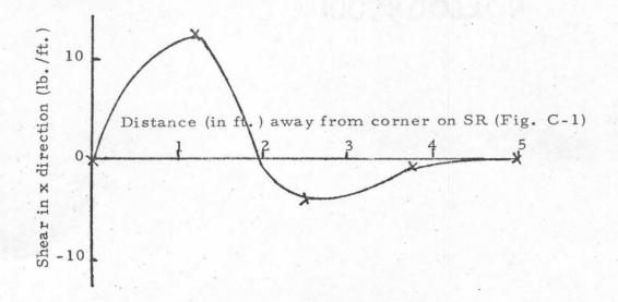
Fig. C-5 Plotting of shear in x direction along SR (Fig. C-1) of problem of a point load on each corner of a sq. plate.
