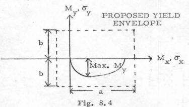
If b in Fig. 8.3 is too small (because the positive  $M_x$  is usually the basic concern, the maximum negative  $M_y$  might exceed the envelope and the plate will break along lines parallel to the x-axis and cracking starts on the top of the plate. A more efficient envelope, it would seem, is of the form shown in Fig. 8.4.
