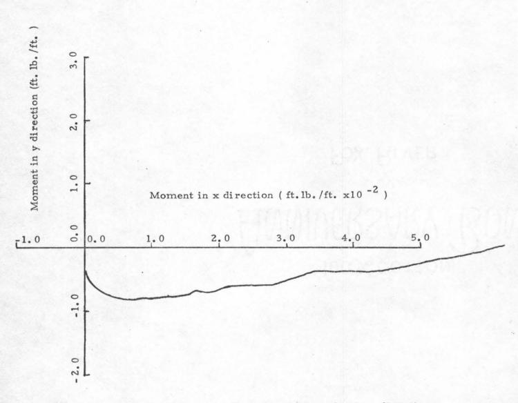
Fig. 8.8 Plotting of moment in x direction against that in y direction along P Q (Fig. 8.2) of point load.
