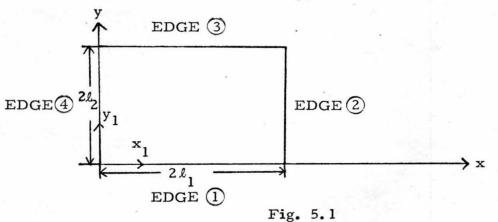
Fig. 5.1 is a rectangular plate with coordinates set up as shown. On the first edge, the  $x_1$ ,  $y_1$  coordinate system coincides with the x-y coordinate system. Expressing the particular solution in the  $x_1$ ,  $y_1$  system and letting  $y_1 = 0$  (coordinates of edge (1)) the following expression for the displacement contribution from the particular solution at the boundary edge (1) is obtained: (derived from eq. (2.9))
