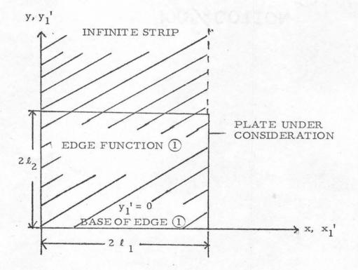
Fig. 4.1. Solution of Edge Function Associated with Edge (1)  $\rightarrow$  0 as  $y'_1 \rightarrow \infty$
