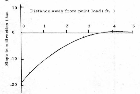
Fig. B-3 Plotting of slope in x direction along PQ
