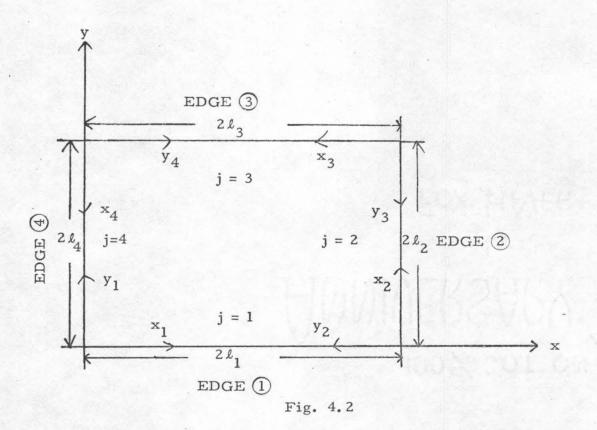
The coordinate axes are set up as shown in Fig. 4.2. The  $x_1, y_1$  axes are chosen such that they coincide with the x, y axes respectively. The different coordinates follow the following relationship:
