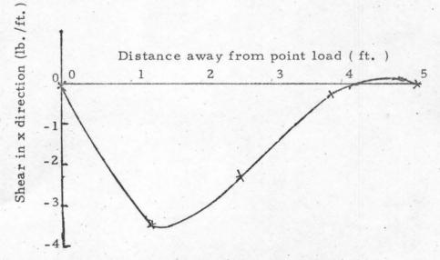
Fig. B-5 Plotting of shear in x direction along PQ.
