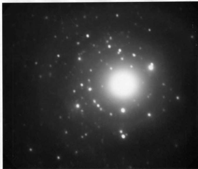
Figure 5-4. Electron diffraction pattern of powdered phosphate rock.
