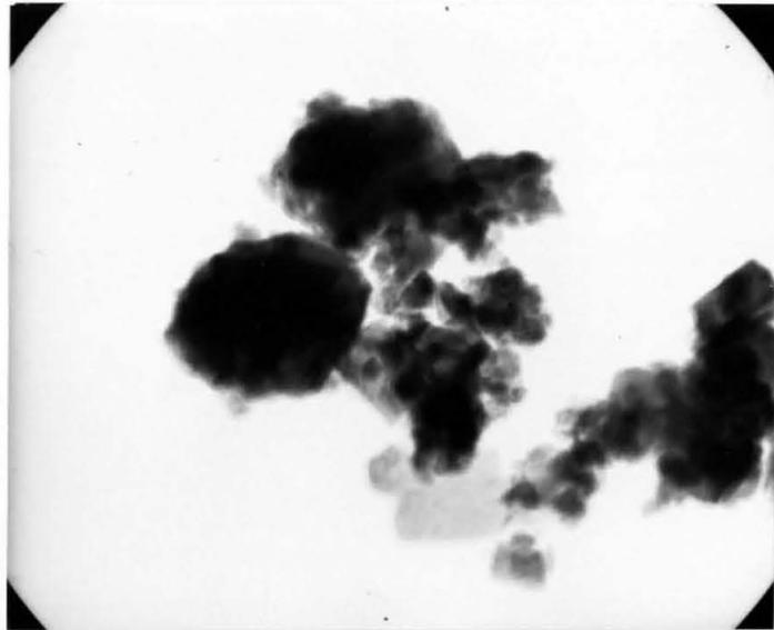
Figure 5-3. Electron micrograph of powdered phosphate rock.
