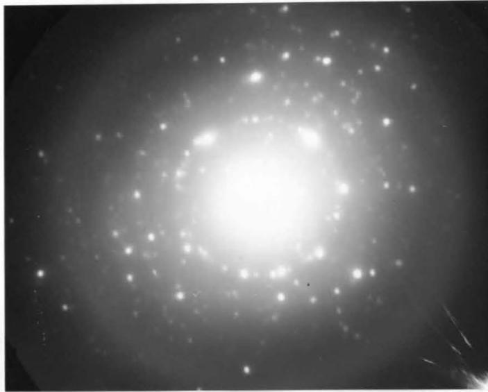
Figure 5-5. Electron diffraction pattern for Run B-4, sample time = -0.0 hours. The sample was equilibrated with 1.0 mM  $\text{CaCl}_2$ , 0.65 mM  $\text{NaHCO}_3$ , and  $3 \times 10^{-4}$  atm  $\text{CO}_2(\text{g})$
