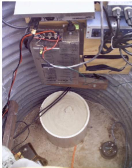
Figure 2.1: A CISN sensor station installed in a “borehole”. Installing and maintaining such stations represents significant investment, but provides exceptional quality.
