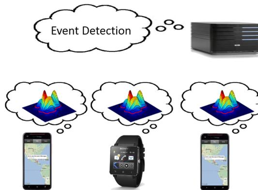
Figure 1.5: An architecture for decentralized event detection: each consumer device runs a client application for modeling its sensor data and transmits pick messages about potential events. A cloud server receives the stream of pick messages, and detects spatial-temporal events.
