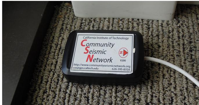
(b) "Phidget USB accelerometer"
