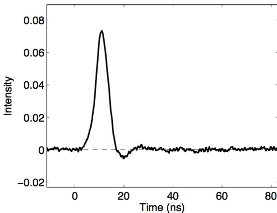
**Figure B.4.** NSI instrument response to scattered laser light, collected on a 2  $\mu$ s window (pulse width: 8 ns).
