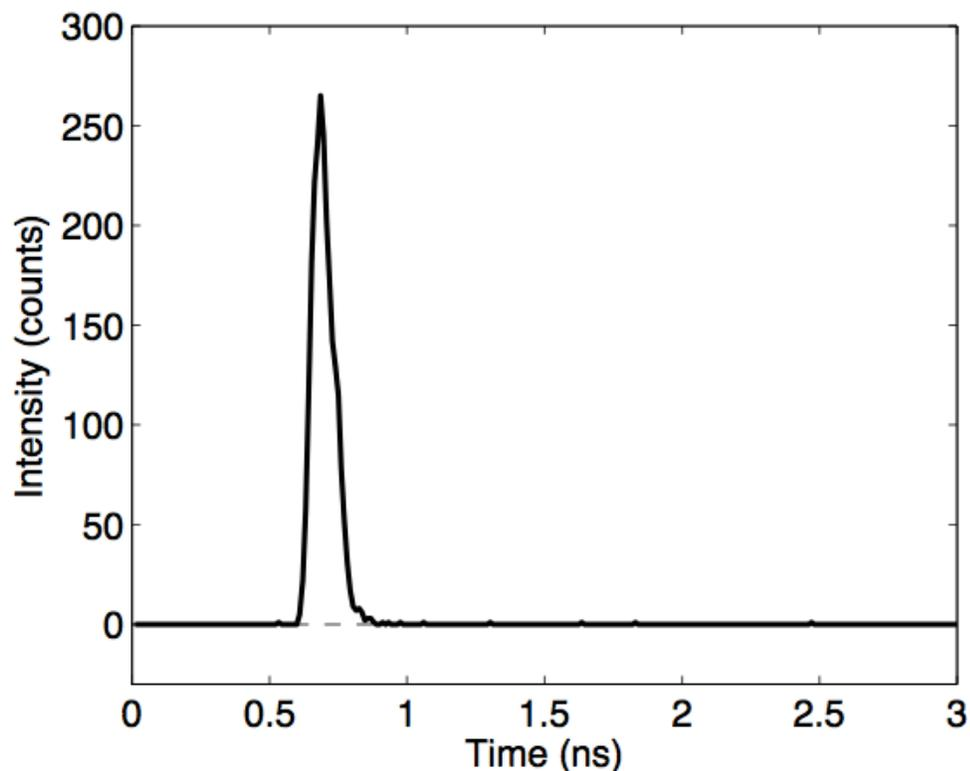
**Figure B.6.** PSI instrument response to scattered laser light, collected on a 5 ns window.
