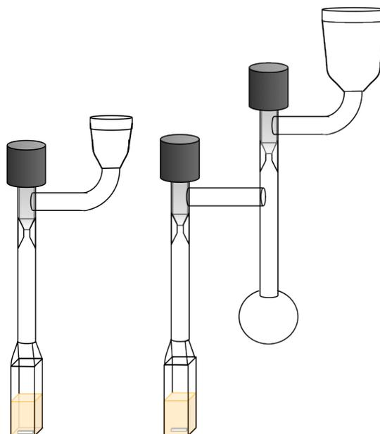
**Figure B.1.** Two high-vacuum cuvettes for laser studies. Left: typical cuvette for flash-quench. Right: cuvette for  $\text{Fe}^{\text{II}}\text{-CO}$  photolysis and rebinding.
