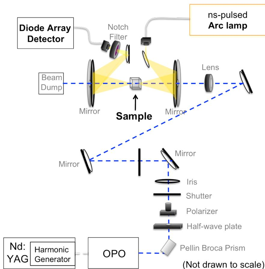
**Figure B.3.** Nanosecond-pulsed multi-wavelength transient absorption setup: NSII.
