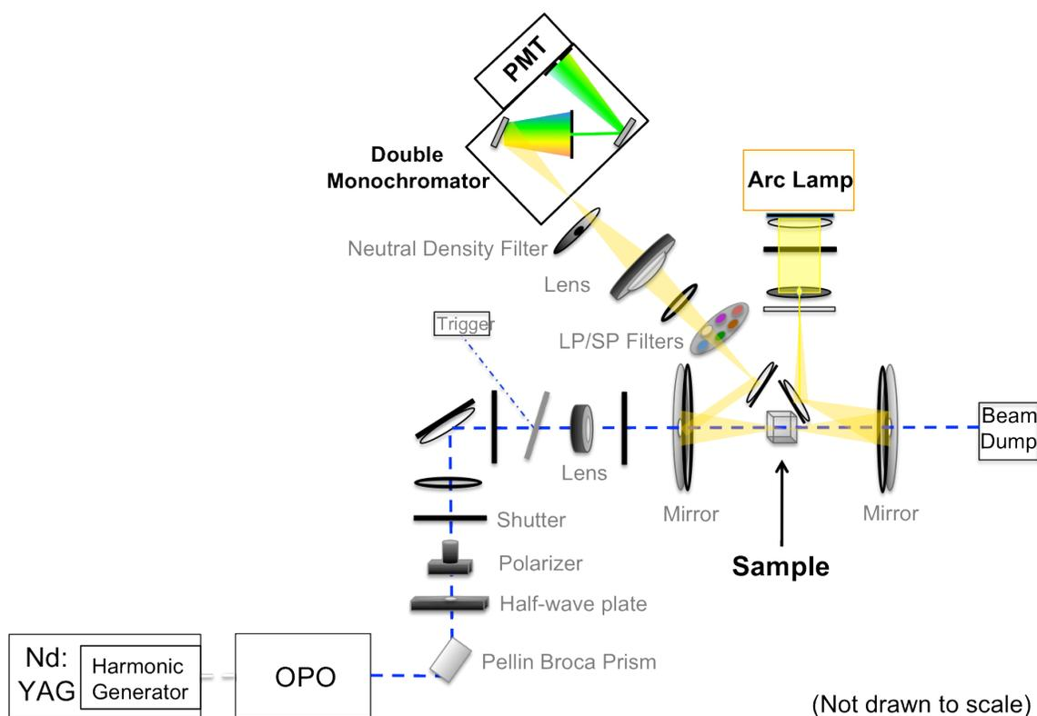
**Figure B.2.** Nanosecond-pulsed single-wavelength transient luminescence and absorption setup: NSI.
