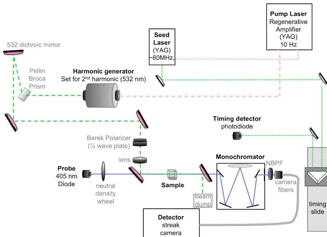
**Figure B.5.** Picosecond-pulsed single-wavelength transient absorption setup: PSI.
