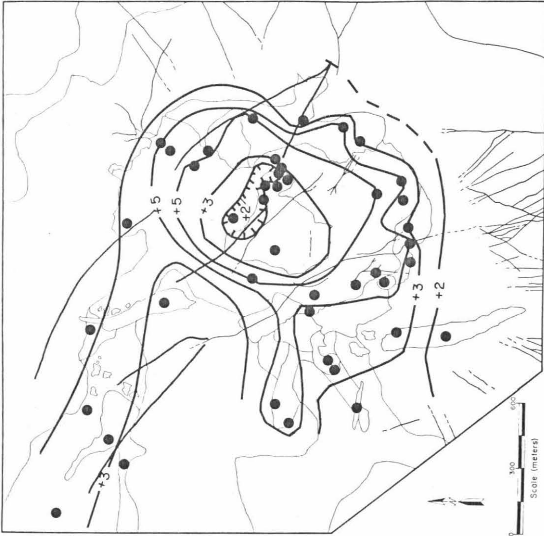
Figure 6-9. Whole rock \delta^{18}O contours of the Stony Mtn. intrusive complex. All samples within the central (hatched) contour have \delta^{18}O < +2 .
