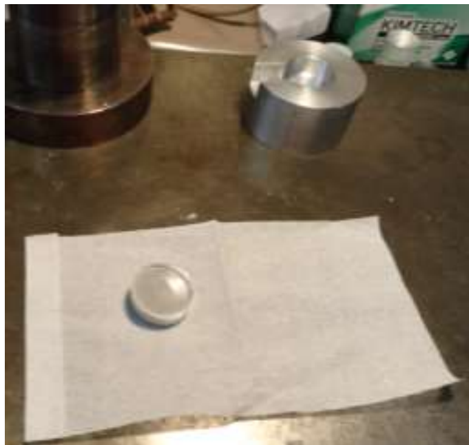
Figure 5.13: Cylindrical alignment holder for aluminum-polymethylmethacrylate wedge configuration.
