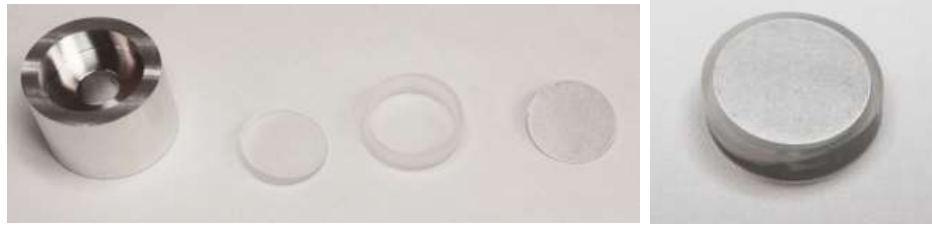
(a) Aluminum alignment cylinder with PMMA wedge and sleeve and aluminum wedge (from left to right). (b) Assembled target configuration with PMMA and aluminum.
