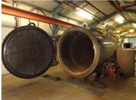
Figure 5.4: Vacuum chamber of Sandia National Laboratories' single stage propellant gun.
