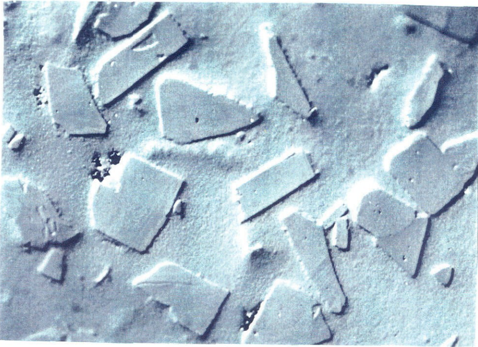
Figure 2.4b Optical micrograph of 15% WC/ Vitreloy® 106 composite. A few small pits are visible, though there is no noticeable reaction layer (400X).
