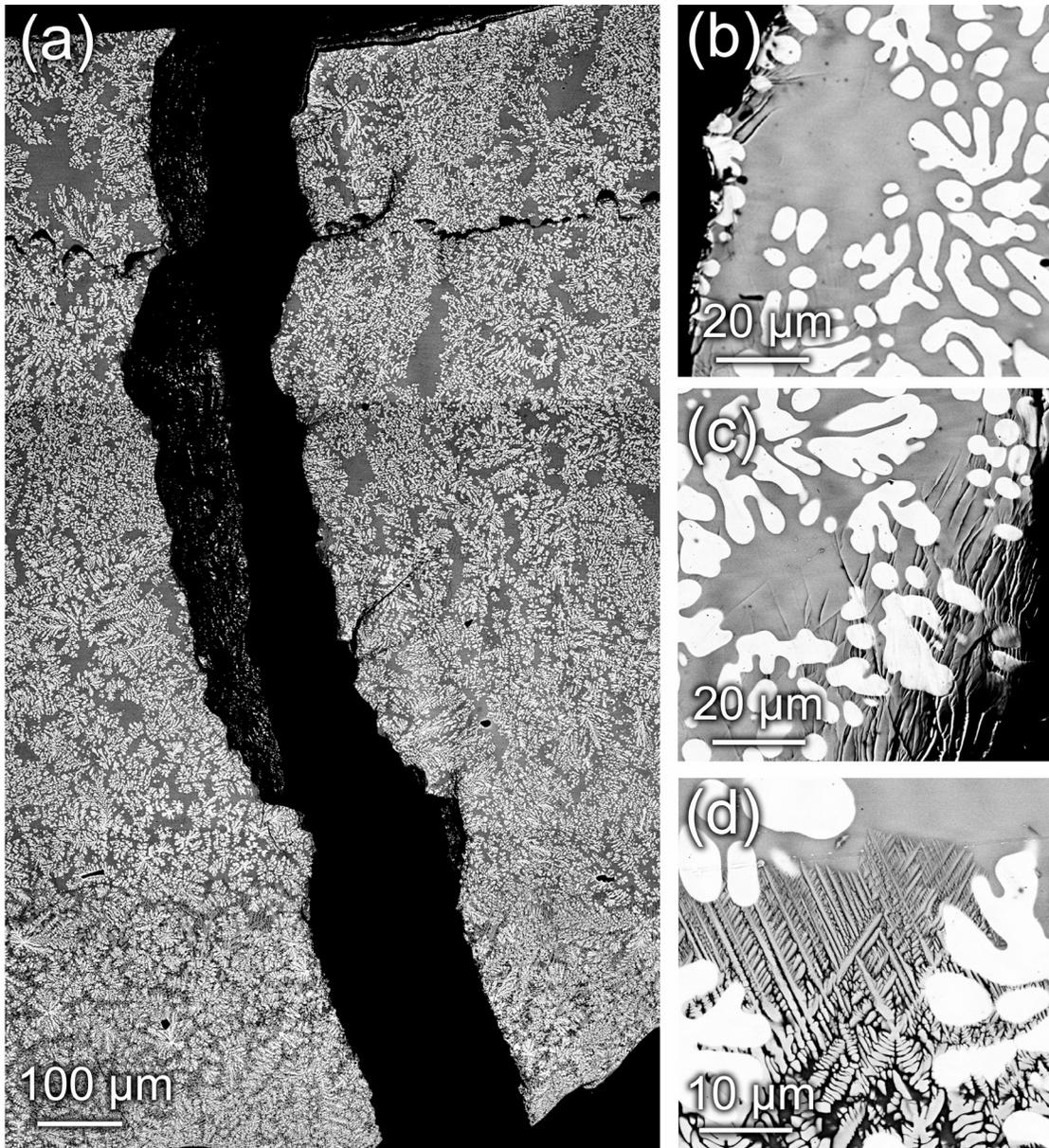
Figure 2-7: (a) A backscattered SEM micrograph showing a fractured specimen of commercially cast LM2. Despite the large, coarse dendrites, other factors (like oxygen content and partial crystallization) make this the most brittle alloy tested. (b) The edge of the crack from a region in (a) demonstrating very little toughness. (c) Another region near the edge of the crack showing that several shear bands have formed. (d) A region where the matrix has crystallized into an unknown brittle phase.
