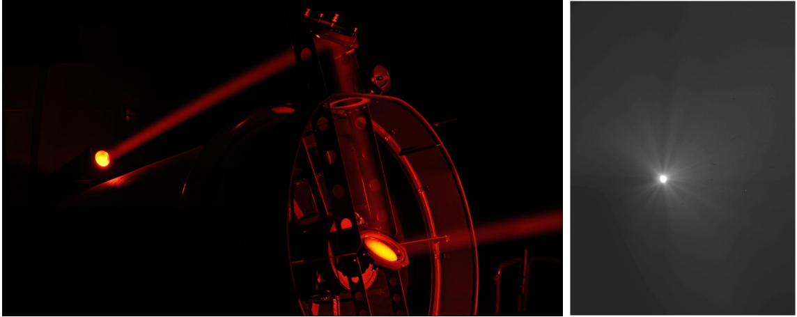
Figure 2.3. Left Panel: The laser periscope assembly with two 10-inch flat mirrors mounted on the top of the telescope tube. This image, taken with a UV sensitive camera shows the beam emanating from the laser projector on the left, reflecting off both the periscope mirrors and propagating into the sky. Photograph by C. Baranec. Right Panel: The beam launched through the periscope along the telescope axis forms a bright star of scattered light in the sky imaged by the existing GRB camera (Cenko et al., 2006) in the U filter.
