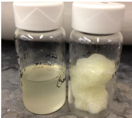
**Figure 3.17** Sticky non-solid PP produced at KFUPM (rt, 8–9 atm propylene) with precatalyst **8** (left) and nonsticky solid PP produced at Caltech (0 °C, 5 atm propylene) also with precatalyst **8** (right).
