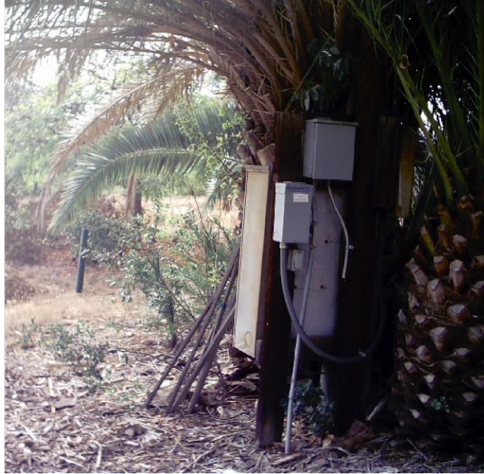
Figure 1.2: A typical CISN installation, in which an Episensor is placed in the ground.
