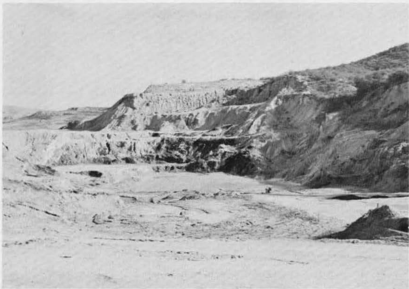
FIGURE 10. View east toward Los Angeles Brick and Clay Products Co. No. 23 clay pit. Black lignite and carbonaceous fire clay, and white sandy fire clay dip 5^{\circ} to 20^{\circ} N. Photo by Mort D. Turner, 1952.
