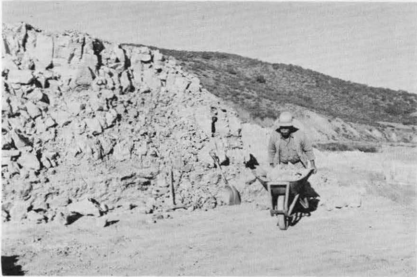
FIGURE 12. Mining sedimentary fire clay in Los Angeles Brick and Clay Products Co. No. 1 clay pit.
