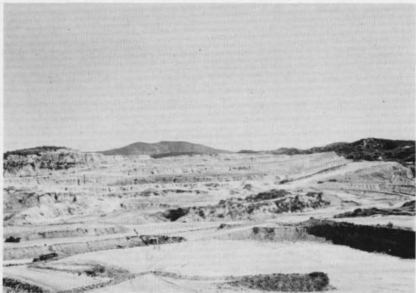
FIGURE 11. View southeast toward Los Angeles Brick and Clay Products Co. No. 1 clay pit. Slate and residual clay are exposed in lower part of pit; white sedimentary fire clay and red and white mottled sandy claystone are exposed on benches in upper part of pit.
