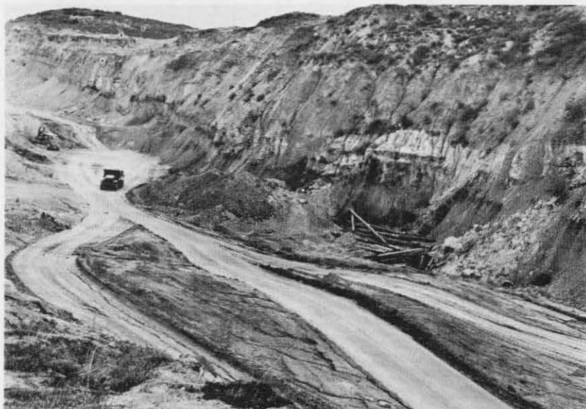
FIGURE 8. View eastward toward south face of Alberhill Coal and Clay Co. West clay pit, showing 4-foot layer of black lignite overlain by white sandy fire clay. Lignite and fire clay pinch out at upper left hand corner of photo. Lignite layer was source of early coal production in Alberhill area. Photo by Charles W. Jennings, 1955.
