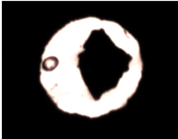
Figure 3.3: (Mg_{0.06}Fe_{0.94})O at 50 GPa in the Synchrotron Mössbauer study. The sample chamber is 150 \mu m across. This study was conducted at 300 K. Ruby sphere is located to the left.
