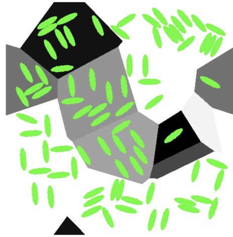
Figure 7.1: Simulated Voronoi microstructure with non-transforming inclusions (green) for anti-plane shear study. (Figure courtesy of D. Sun.)
