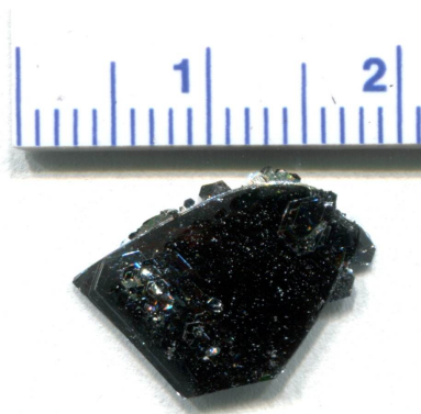
Figure 4.4. Photograph of a large \text{WSe}_2 crystallite grown by CVT using \text{WO}_2\text{Cl}_2 transport agent without any extrinsic doping source. Numbered demarcations on the ruler are centimeters.
