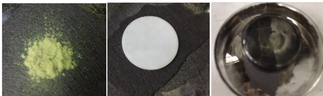
Figure 5.1: (a) \text{Pt}(\text{acac})_2 powder on porous carbon paper, (b) as pressed \text{CsH}_2\text{PO}_4 pellet, (c) \text{Pt}(\text{acac})_2 powder|carbon paper|electrospayed \text{CsH}_2\text{PO}_4 | \text{CsH}_2\text{PO}_4 pellet|electrospayed \text{CsH}_2\text{PO}_4 |carbon paper| \text{Pt}(\text{acac})_2 powder in a Petri dish.
