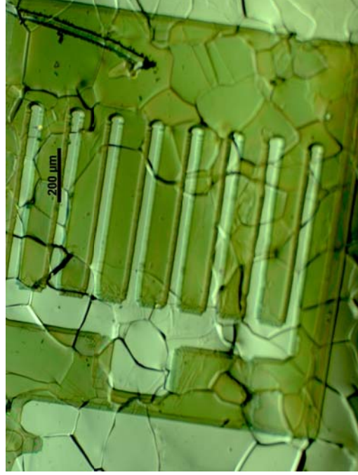
Figure 3.10. Optical micrograph images of heterostructures being patterned.
