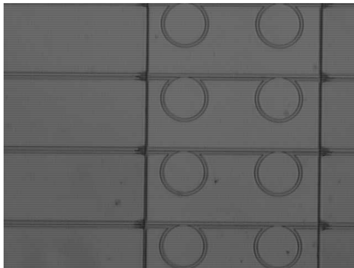
Figure 5.4: An overhead image of the dual disk resonators within a dual flow microfluidic channel
