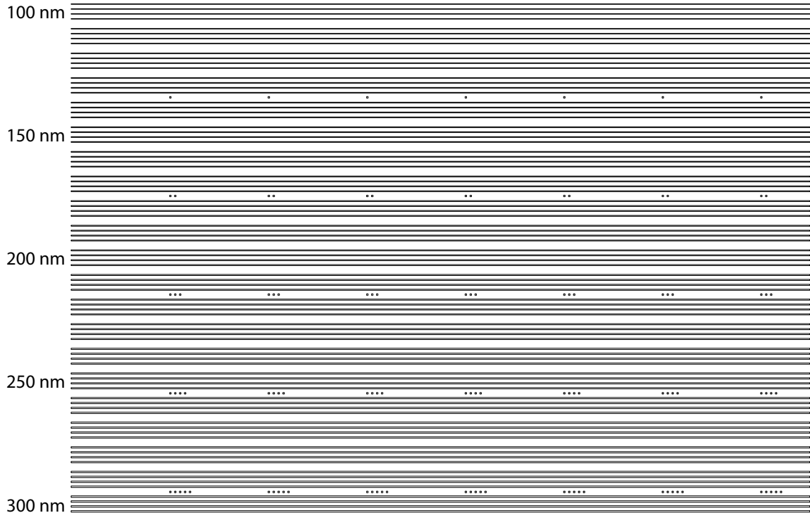
Figure 3.14: Etch test pattern. The etch test pattern used for etch optimization of the silicon nitride nanobeams. The pattern consists of groups of four trenches a full FoV long. The trench width varies over each group of four with the first group having a width of 100 nm, the last having a width of 300 nm with the width increasing by 10 nm each group. The squares separating each set of four groups provide a count allowing easier determination when imaging (SEMing).
