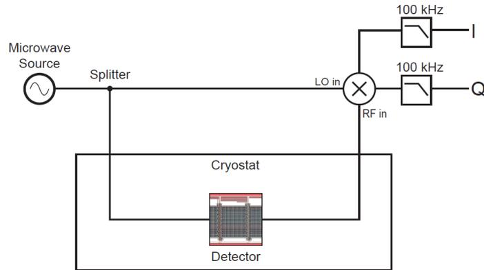
Figure 2.1: Measurement setup. A frequency tone generated by a microwave source is split, with one component traversing the transmission line near the detector pixels, and recombined by a mixer to retrieve orthogonal components of the signal, which are used to calculate amplitude and phase information.
