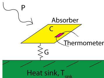
Figure 1.1: Schematic diagram of a bolometer pixel. A thermometer measures the temperature change associated with a change in incident power  $P$  on the absorber with heat capacity  $C$ . Heat escapes to the substrate via thin legs with combined thermal conductance  $G$ .
