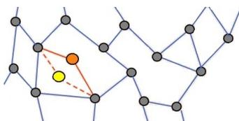
Figure 1.4: Two level systems, in which an atom may quantum tunnel between two local minima in potential energy, are hosted in a thin amorphous surface layer on the crystalline substrate. They introduce excess noise in the position of the resonant frequency in a resonant circuit.
