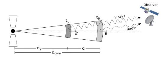
Figure 7.1: Schematic of the model used in the interpretation of the time lag between the radio and gamma-ray emission. The central engine in the far right launches a jet in which moving disturbances propagate away at speed  $\beta$ . A moving disturbance (shaded area) is depicted at two times:  $t_{\gamma}$  at which gamma-ray emission peaks and  $t_r$  for the peak of the radio emission when crossing the radio core. All the relevant distances have been indicated.
