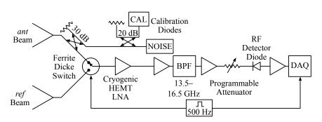
Figure 2.3: The Ku-band receiver. Credit: Richards, J. L., et al. 2011, ApJS, 194, 29, reproduced by permission of the AAS.
