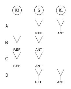
Figure 2.4: Illustration of the double switching procedure. The circles at the top of the figure represent the field containing the source (S), and the two reference fields used to subtract atmospheric contributions (R1 and R2). A flux density measurement consists of four segments called A, B, C and D. For each one the positions of the antenna and reference fields are indicated with respect to the sky fields.
