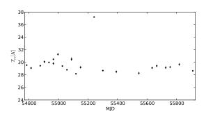
Figure B.1: Receiver noise temperature measured with a hot/cold test. Excluding the February 2010 outlier the mean value is  $T_{\rm rx} = 29.4 \pm 0.2$  K.
