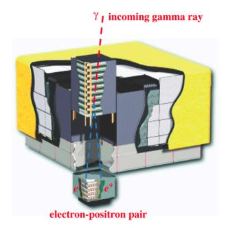
Figure 2.25: Schematic diagram of the LAT. Its dimensions are  $1.8 \text{ m} \times 1.8 \text{ m} \times 0.72 \text{ m}$ . It consist of a  $4 \times 4$  array of 16 modules for the converter-tracker and calorimeter. An anti-coincidence detector covers the converter-tracker array. Credit: Atwood, W. B., et al. 2009, ApJ, 697, 1071, reproduced by permission of the AAS.
