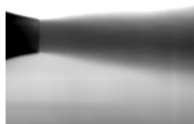
Figure F.7: Averaged dye visualization for T = 1500 and \tau = 0 s. Phase-averaged frame consists of 53 frames are stacked.
