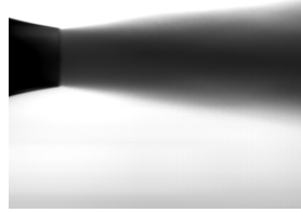
Figure F.1: Averaged dye visualization for T = 1300 and \tau = 0 s. Phase-averaged frame consists of 51 frames are stacked.
