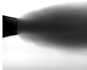
Figure F.4: Averaged dye visualization for T = 1300 and \tau = 8 s. Phase-averaged frame consists of 105 frames are stacked.
