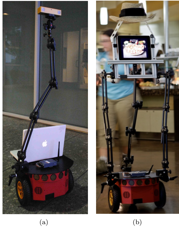
Figure 4.7: (a) The original form factor of the Pioneer 3-DX. The single arm with mounted stereo camera was essentially invisible from many vantage points. Mounted Bumblebee camera was not prominent enough to produce saliency. (b) The current form factor of the Pioneer 3-DX. Notice the inclusion of multiple camera arms (to produce the impression of a human like volume), an 80/20 “face” with iPad (for motion and audition purposes). The sun hat protects the robot from the bright overhead lights.
