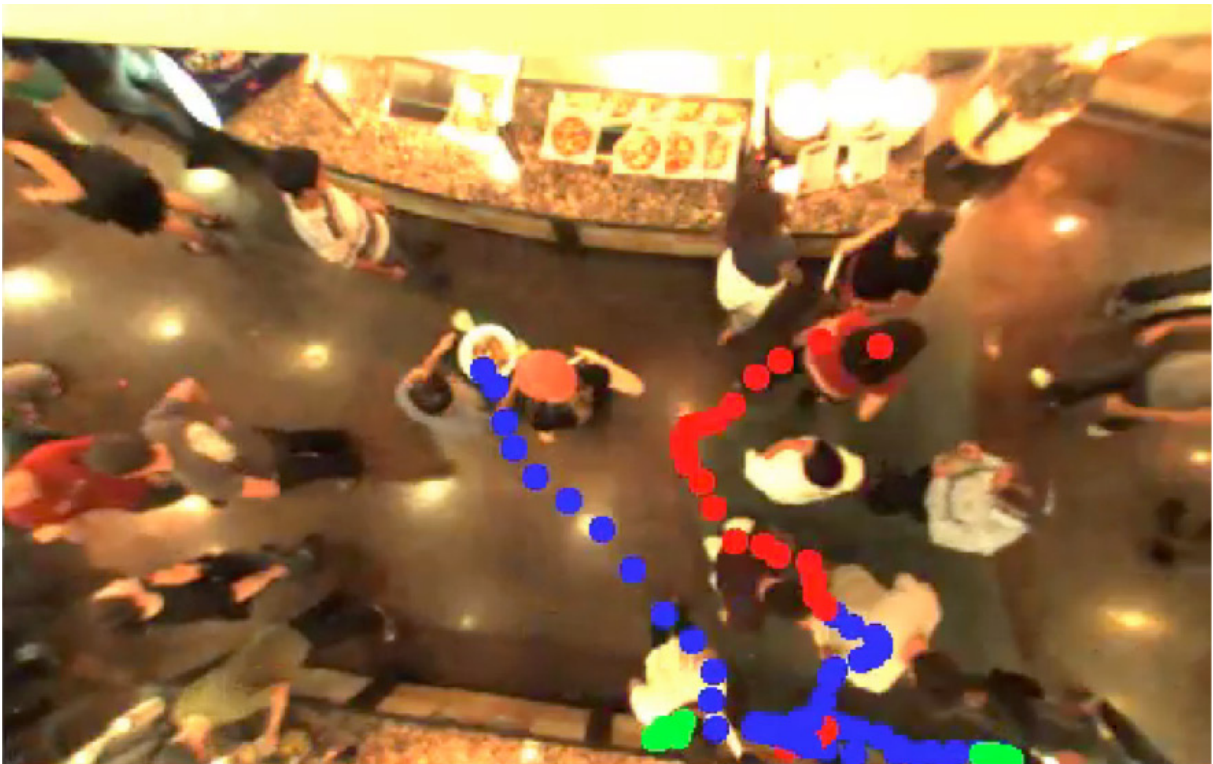
Figure 3.1: An example trajectory of a cafeteria patron. The trajectory was hand labeled and segmented; blue dots are part of the nominal trajectory (modeled with the kernel function k = k_{linear} + k_{matern} + k_{noise} , as in Section 2.3.2.3), green dots are goals (see Section 3.1.2.2), and red represents interaction between agents (see Section 3.1.3)
