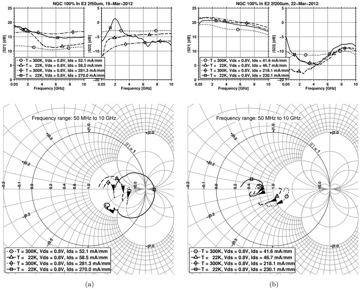
Figure 6.8: Measured, cryogenic  $S_{22}$  and  $S_{21}$  of the 2f50 and 2f200  $\mu\text{m}$  NGC 100% transistors. The measurements are de-embedded to the edge of the devices which are the same devices as those presented in Section 6.2.
