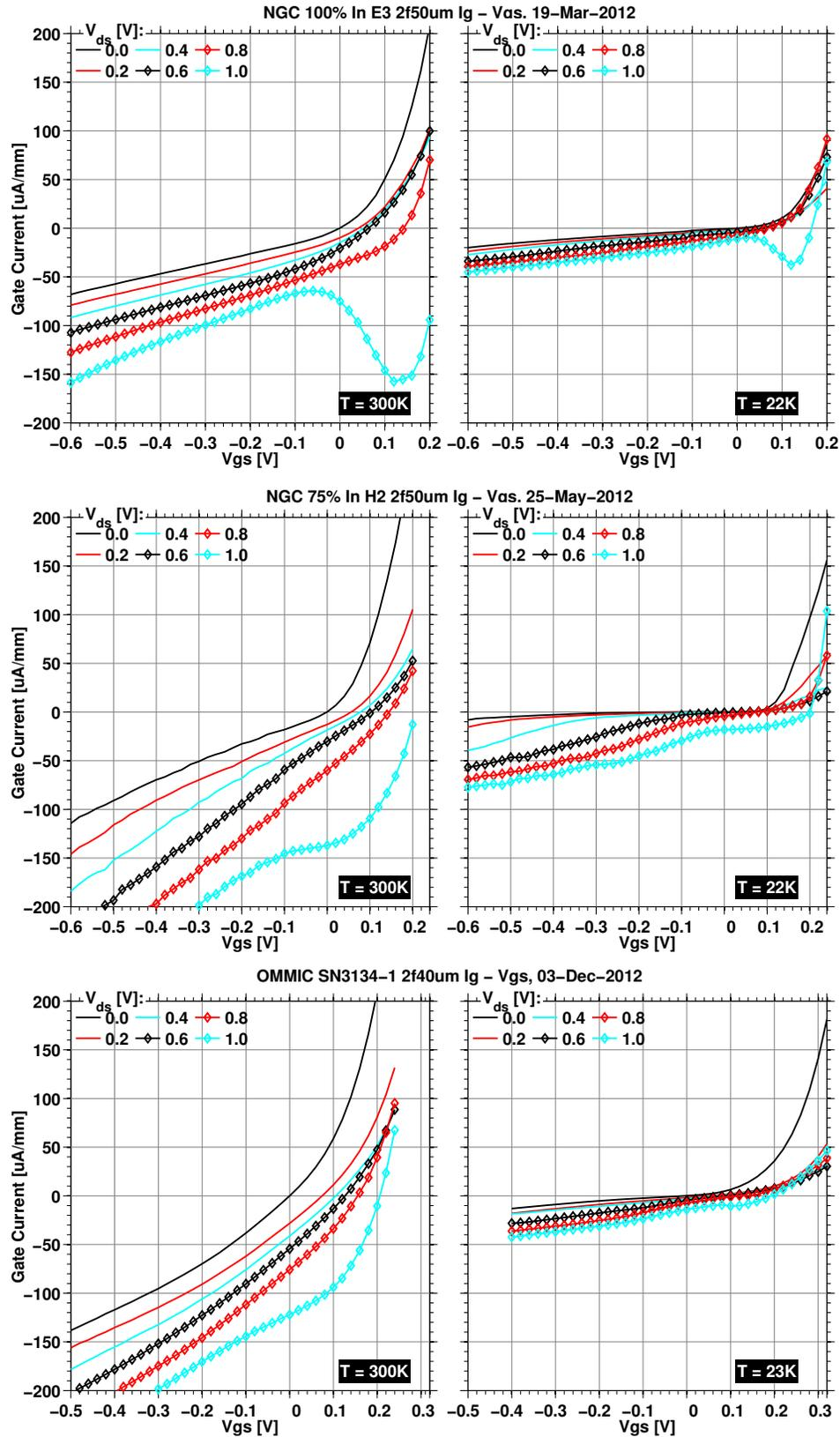
Figure 6.6: Measured  $I_{GS} - V_{GS}$  of NGC 100% 2f50  $\mu\text{m}$  (top), NGC 75% 2f50  $\mu\text{m}$  (middle), and OMMIC 2f40  $\mu\text{m}$  devices
