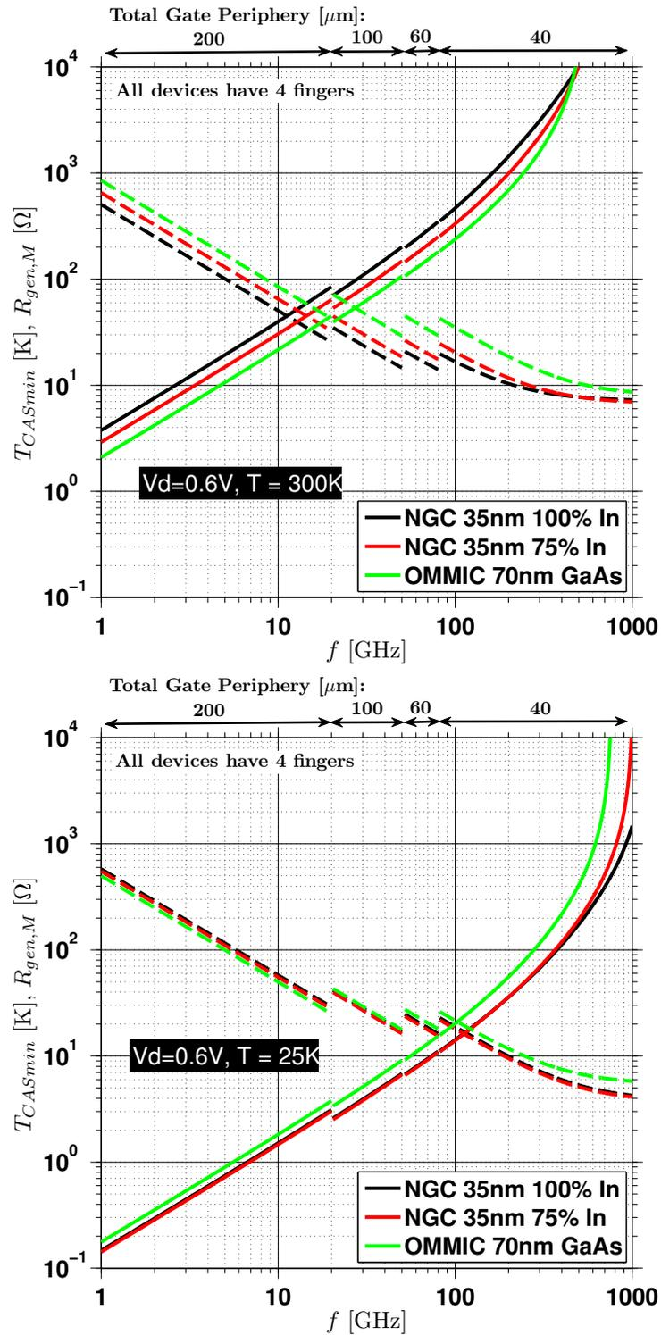
Figure 6.16:  $T_{CASmin}$  (solid) and  $\Re\{Z_{gen,M}\}$  (dashed) of the three processes versus frequency at 300 K (top) and 25 K (bottom).  $I_{DS} = 100, 150$  mA/mm at 300 K and  $I_{DS} = 25, 40$  mA/mm at 25 K for NGC and OMMIC devices, respectively.
