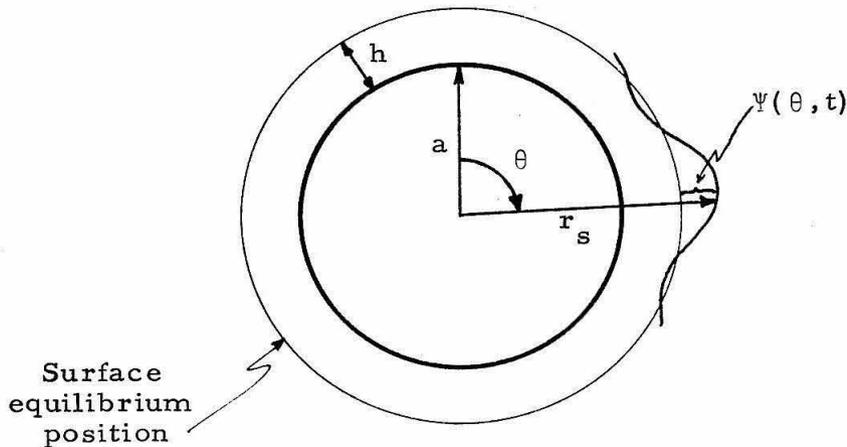
Figure A-1. Definition of parameters describing the free-surface waves.
