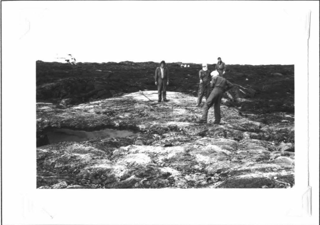
**Figure 5-2a: Photograph of lava tube monitoring.** This photograph shows HVO staff members collecting a lava sample out of a skylight on the Wahaula lava tube. A cable with a hammer head attached to its end is dropped into the skylight. It is pulled out after the hammer head has been immersed in the lava stream. Note the incandescent lava coated hammer head in mid-air. Also note the helicopter. Usually helicopters were not available and all gear was man-ported to (and from) the skylights.
