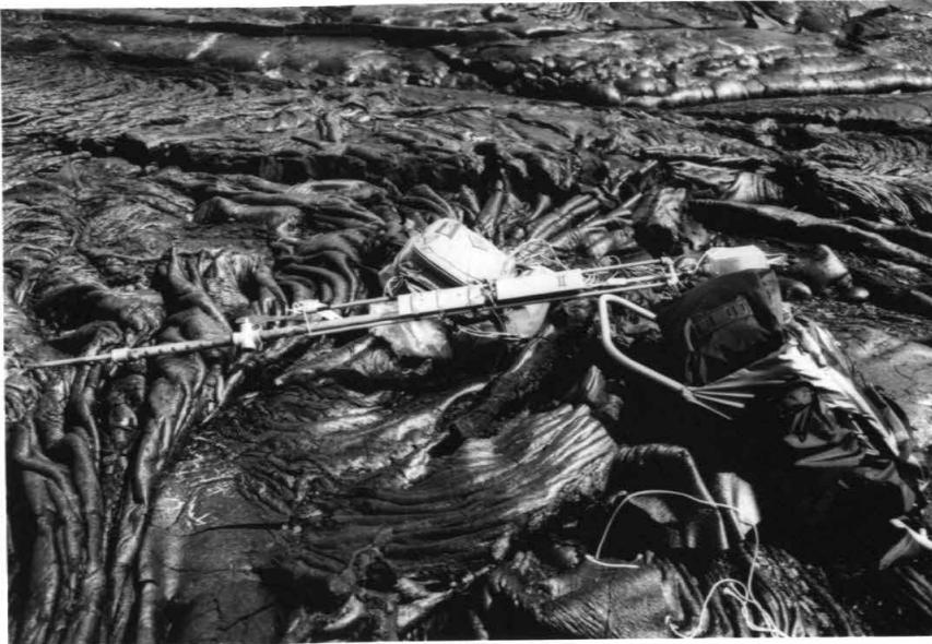
**Figure C-6: Photograph of Lava Lance in the field.** The data logger and power systems are in the small backpack and the laptop and repair kit are in the large backpack.
