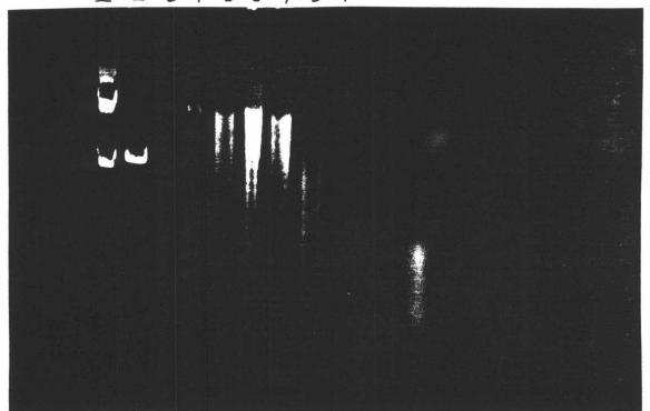
1.2% agarose gel of Lysobacter DNA digests stained with ethidium bromide. Lane 1 is 0.85ug of pBR322; lane 2, lug of pBR322 cut with HincII; lane 3 through 6, 15ug of Lysobacter DNA cut with BamHI, SphI, SalI and NruI, respectively; lane 7, 5ug of Lysobacter DNA.
