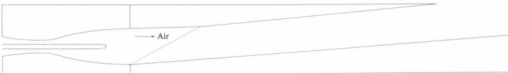
Figure 2.1 Side view of wind tunnel test section
