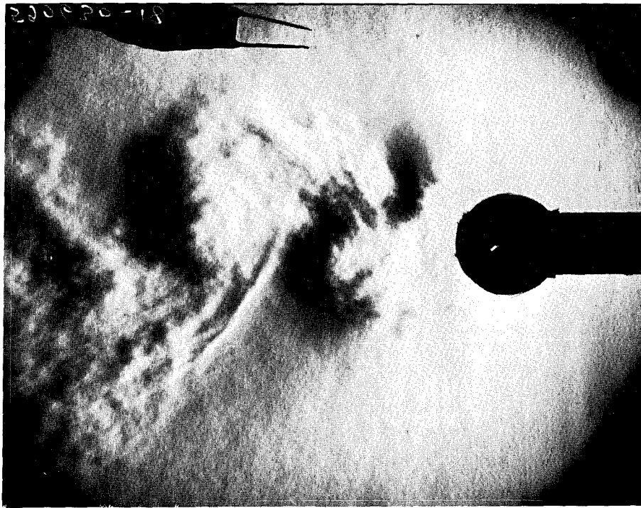
Fig. 29 - Typical Schlieren flash ( 4\mu\text{sec} ) photographs of wake ; M_1 = 0.55
