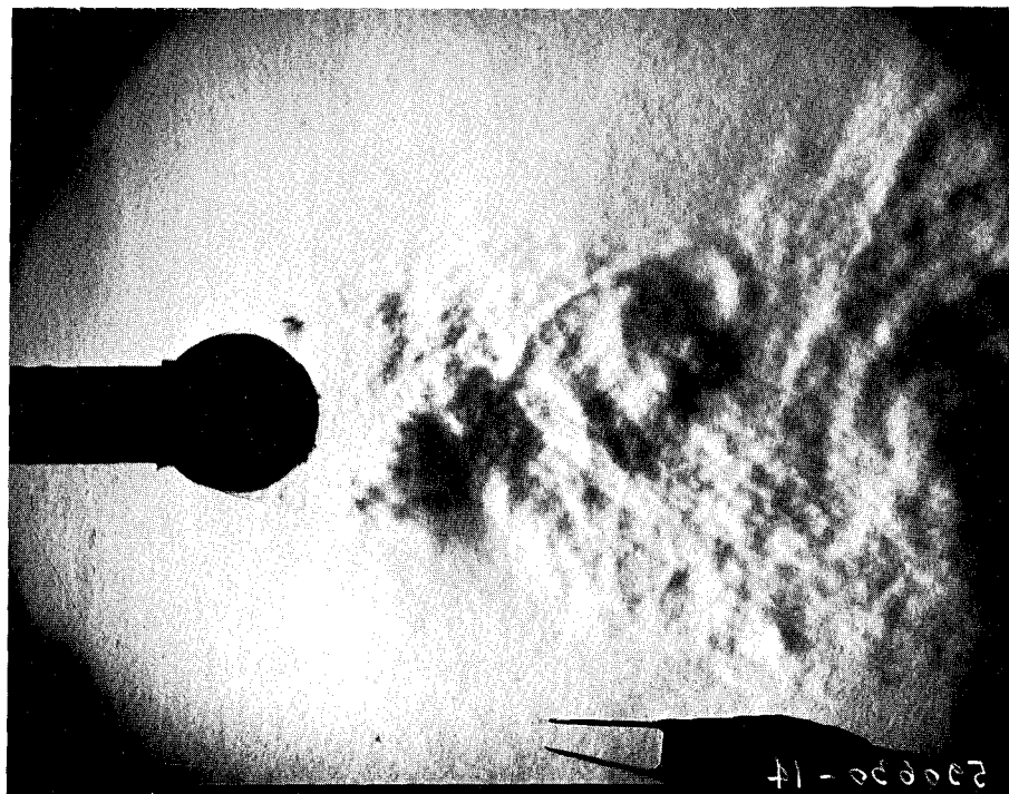
Fig. 28 - Typical Schlieren flash ( 4\mu\text{sec} ) photographs of wake ; M_1 = 0.50
