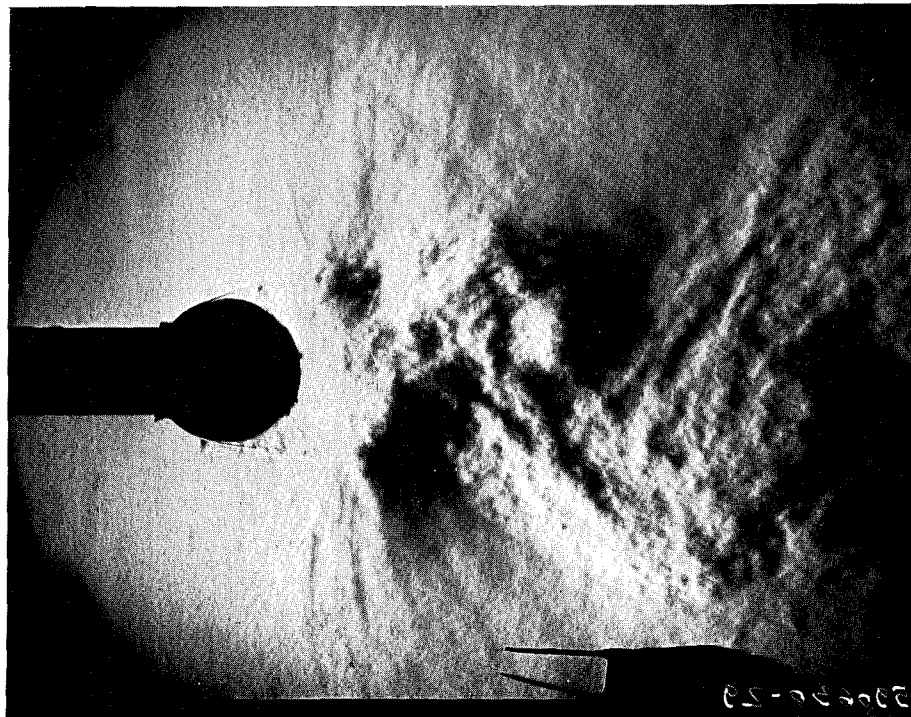
Fig. 30 - Typical Schlieren flash ( 4\mu\text{sec} ) photographs of wake ; M_1 = 0.60
