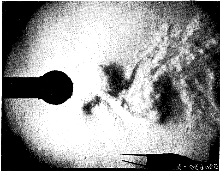
Fig. 26 - Typical Schlieren flash ( 4\mu\text{sec} ) photographs of wake ; M_1 = 0.40
