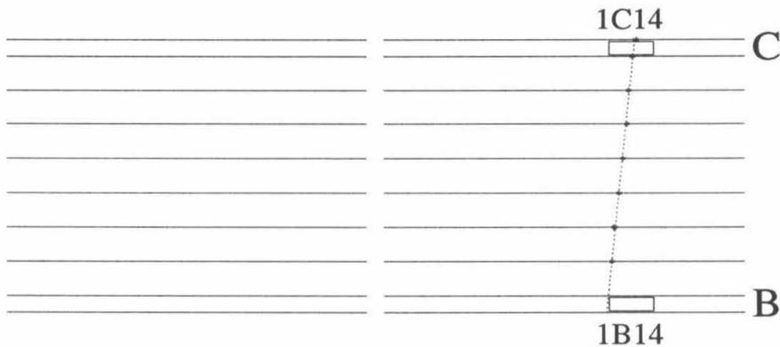
**Figure 4.31:** An FMT candidate which is a stopping muon. Six of the eight final FMT candidates have similar signals in both waveforms and streamer tubes, indicating that they are stopping muons. For simplicity, we only show the streamer tube wire view, in which a dot indicates a hit wire, a box indicates a fired scintillator counter and the dashes are best-fit muon tracks.
