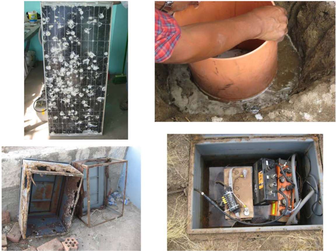
Figure C.5 Photos show a few field challenges such as water filling boxes and holes, solar panels not generating sufficient power, and equipment which gets damaged, malfunctions, or is stolen.
