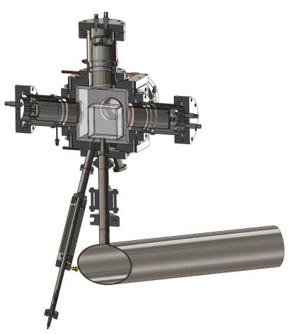
Figure 8.17. This CAD drawing shows a cross section of the UCNb experiment in one of the proposed 2012 geometries. Inside is shown the  $CaF_2$  scintillator with a MgF<sub>2</sub> coating.
