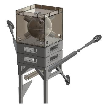
Figure 9.1. This drawing shows a cartoon of a possible upgrade of the UCNb experiment. There are eight PMTs that lie on the faces of a virtual icosahedron that lay on the outer spherical vacuum jacket.
