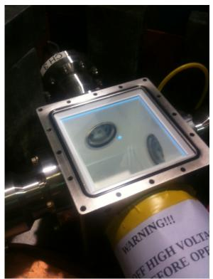
Figure 8.2. This photo shows the  $MgF_2$  polystyrene scintillator box assembled and placed inside the integrating cube. The top is on top of the box showing the insert hole for the insertable source.
