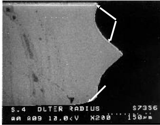
Figure 2.8: Cross-section of screen grid webbing after 8200-hour wear test.
