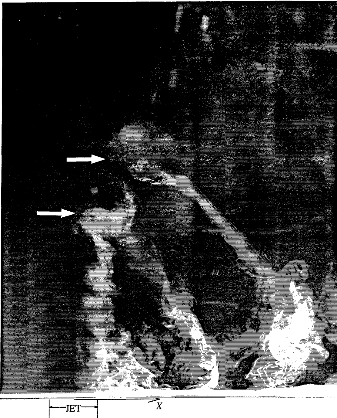
FIGURE 5.10: Two wake vortices attached at the trailing edge of the jet. VR = 5.8 . Re_{cf} = 3800 . Z_{sw}/D_j = 0+ .
