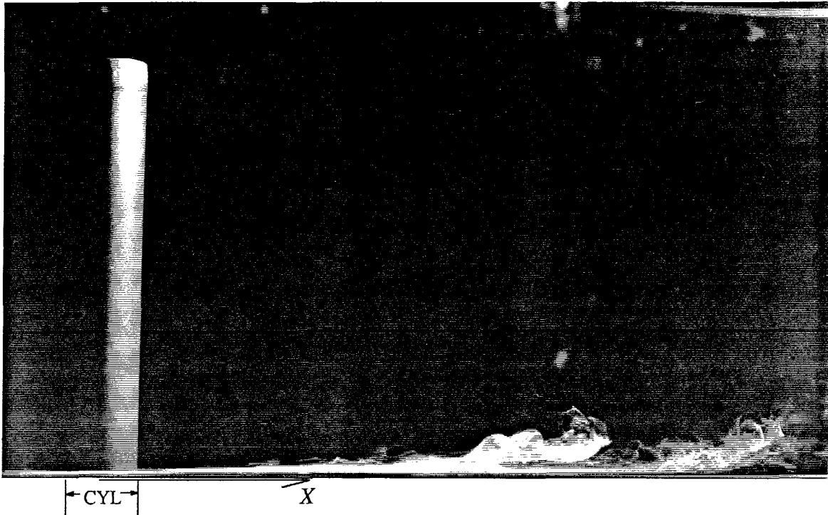
FIGURE 5.18: Side view of flow about a circular cylinder. AR = 6 . Re_{cf} = 3800 . Z_{sw}/D_j = 0+ .
