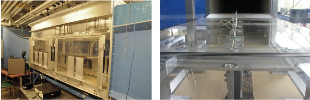
Figure 2.1: (Left) The test section, as shown from the outside, with the direction of flow from left to right. (Right) The plate seated on its supports within the test section, with the direction of flow from bottom of the image to top. The roughness elements and diagnostics traverse are both visible, along with both the acrylic walls and adjustable ceiling of the test section.
