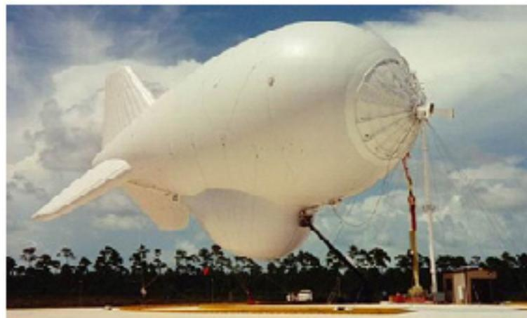
Figure 1.4. Tethered aerostat (courtesy of ILC Dover).
