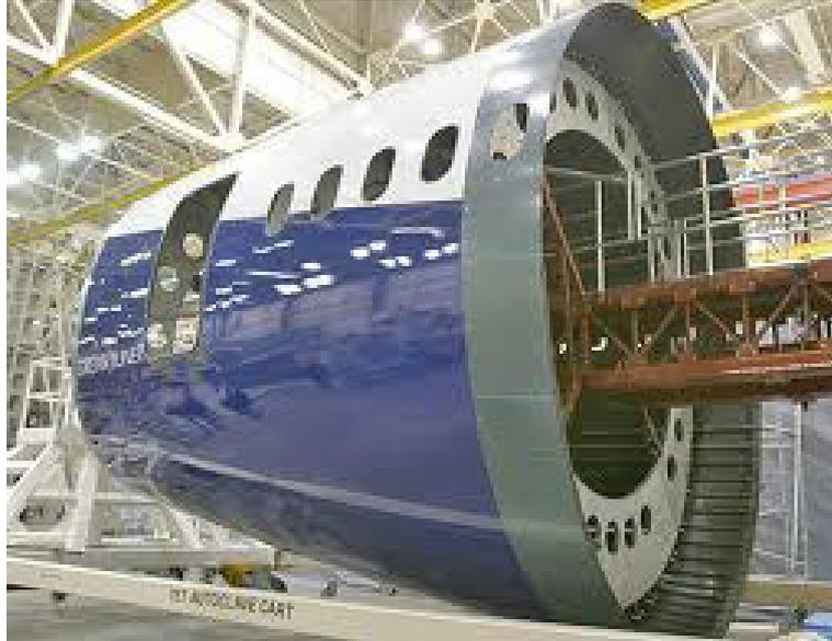
Figure 1.1. Carbon fiber composite fuselage section (courtesy of Boeing).
