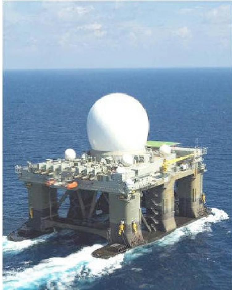
Figure 1.3. Sea-based inflatable radome (courtesy of ILC Dover).
