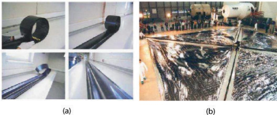
Figure 1.2. Composite deployable booms: (a) Snapshots during deployment, and (b) solar sail unfolded by four deployable booms (courtesy of DLR).
