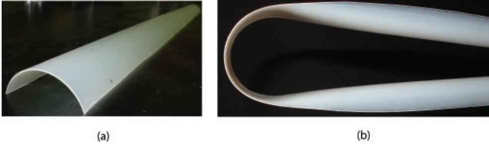
Figure 4.2. Tape-spring made of LDPE having a radius of 19 mm and a subtended angle of  $150^\circ$ : (a) deployed and (b) folded.
