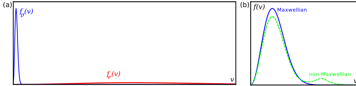
Figure 1.2: a.) Velocity distribution functions f_{p+}(v) and f_{e-}(v) for ions and electrons, respectively, that have equilibrated at the same temperature. b.) Even within a single species, if there is a source of heating but insufficient collisions to distribute that energy among all the particles, a non-Maxwellian distribution may arise, and the temperature would not be well defined.
