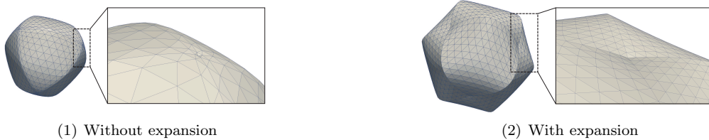
Figure 5.16: Zoomed-in results near the boundary of \mathcal{M}_X using both of the simple method and the expansion method. Concavity is better preserved using the latter method.
